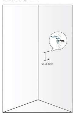
(2) Secure the mounting bracket to the wall (pay attention to the orientation of the mounting bracket). After adjusting the installation position, use two Philips pan head screws to secure the mounting bracket to the wall.
