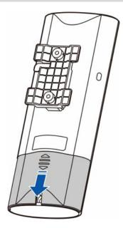
(2) Connect one end of the Ethernet cable to the LAN/2.5G/PoE port, and press the Ethernet cable into the Ethernet cable holder.
