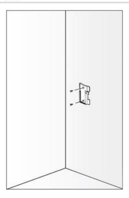
(3) Align the slots on the back of the AP with the square feet on the mounting bracket, and slide the AP down into the mounting bracket slowly to ensure that the AP is secured.
