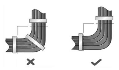
Cables not to be assembled or remaining parts of cables should be folded and placed in a proper position of
