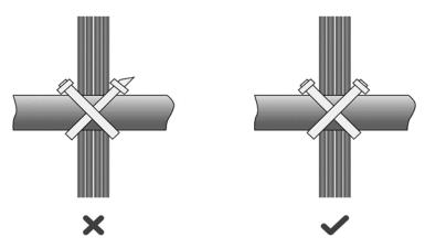
• When cables need to be bent, you should first bundle them up, as shown in <u>Figure 7-5</u>. However, the buckle cannot be bundled within the bend area. Otherwise, considerable stress may be generated in cables, breaking cable cores.
